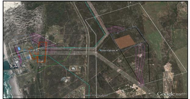
**Figure 2:** Weskusfleur substation - The two sites (Alternative 1 and Alternative 4) that were considered in this study – site 1 is the GIS small full colour blue block and site 4 is the AIS brown full colour block. The blue rectangular bock at site one not coloured in is to show if an AIS was to be considered at site one with the purple
